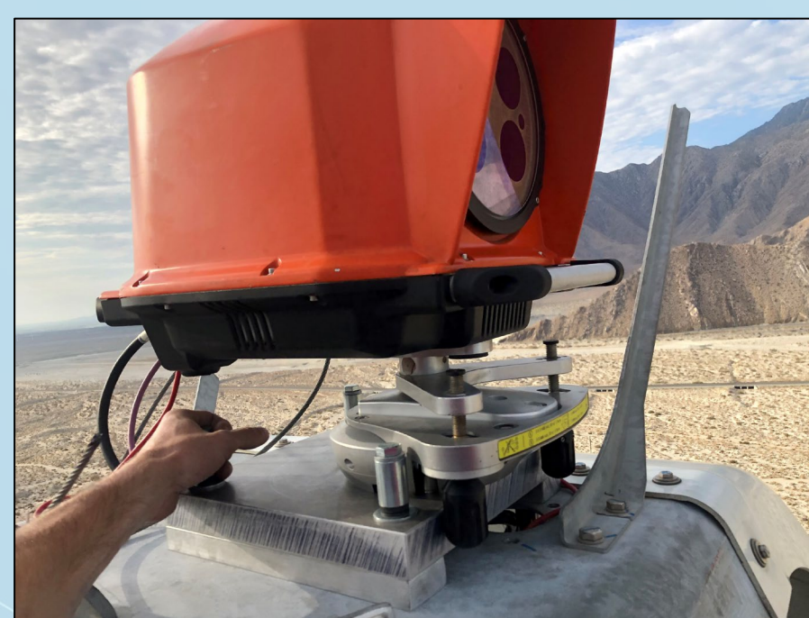
Figure 4: Four-beam NML lidar installed on the test turbine.
