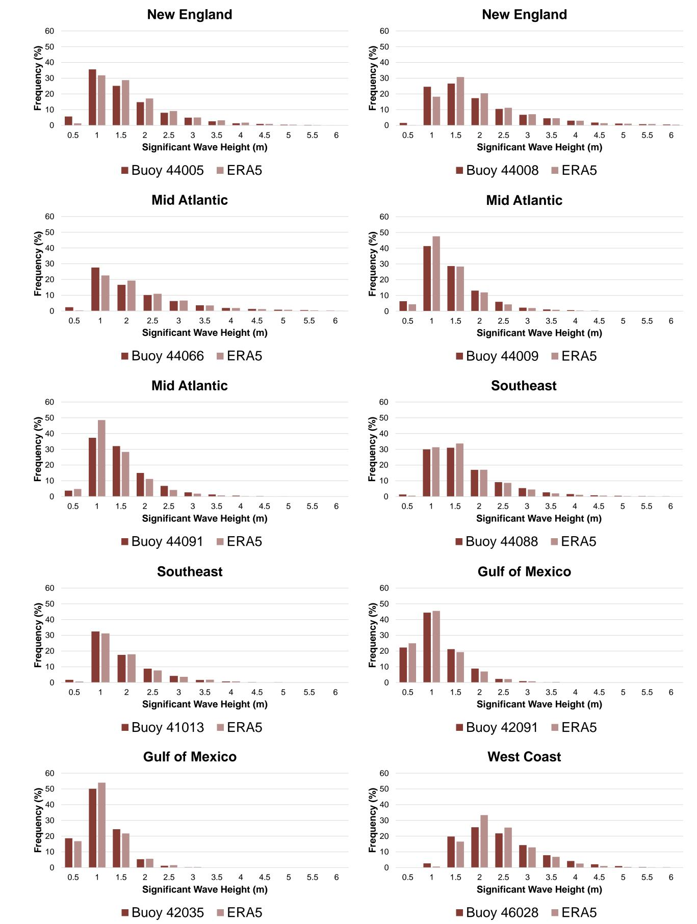
waves and swell) parameter against concurrent National Data Buoy Center (NDBC) buoy measurements off the east and west coasts of the USA and against the FINO3 mast in the North Sea. The average biases in model performance are quantified as is model performance by region and with varying proximity to shore.
