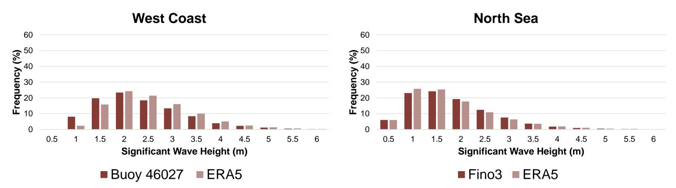
The ERA5 and measured buoy SWH frequency distribution graphs for a subset of the study areas shown above illustrate the sensitivity of the modeled SWH distributions around the 1.5-2.5 m SWH that are relevant for crew transport vessel operation for offshore wind energy. The graphs further illustrate the regional differences in SWH frequency distributions that will impact estimates of site access loss and turbine availability.
