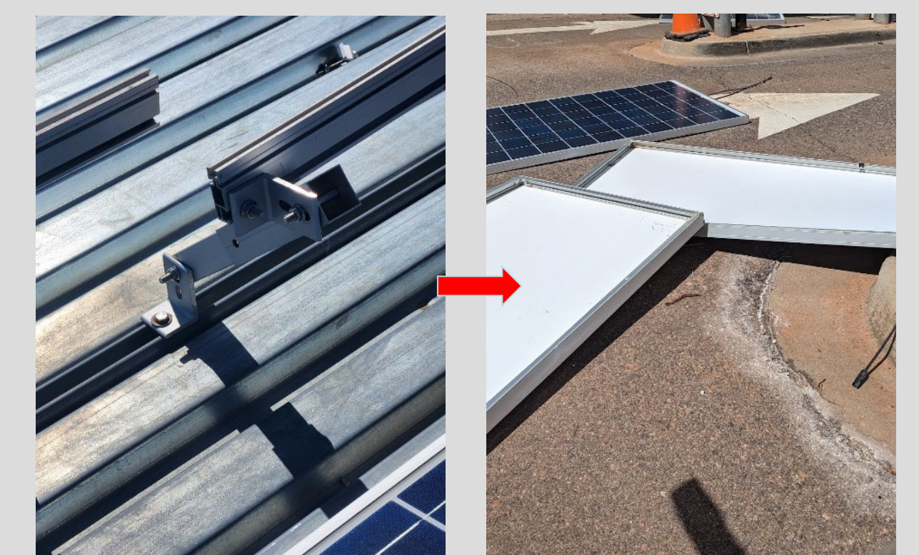
Mounting strength insufficient → bent bracket
