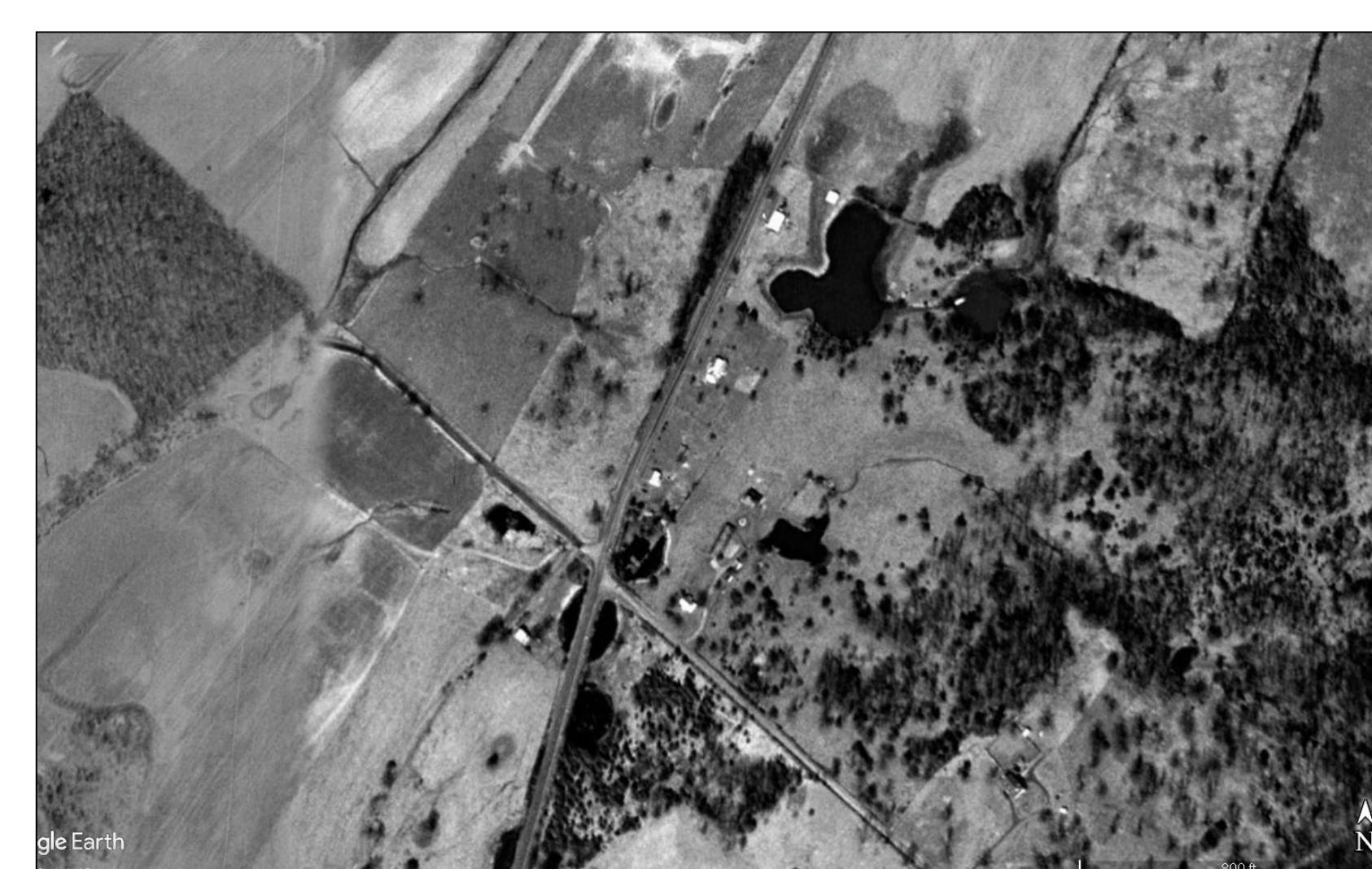
Survey area during period of wet weather showing flooded sinkholes
