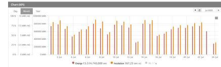
Figure 5.2: Daily energy production and insolation registered in Girasol PV plant during July 2023. A SAL was over Girasol PV Plant on July 21st and 22nd 2023, the energy output was around 7% to 8% smaller than a normal. Smaller data reported on the other days were caused by strong clouds and rainy days.
