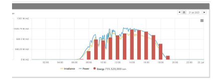
Figure 5.4: Daily energy production, irradiance and power registered in Girasol PV plant during July 2023. On the top July 7 th , 2023. On bottom July 21st, 2023.
