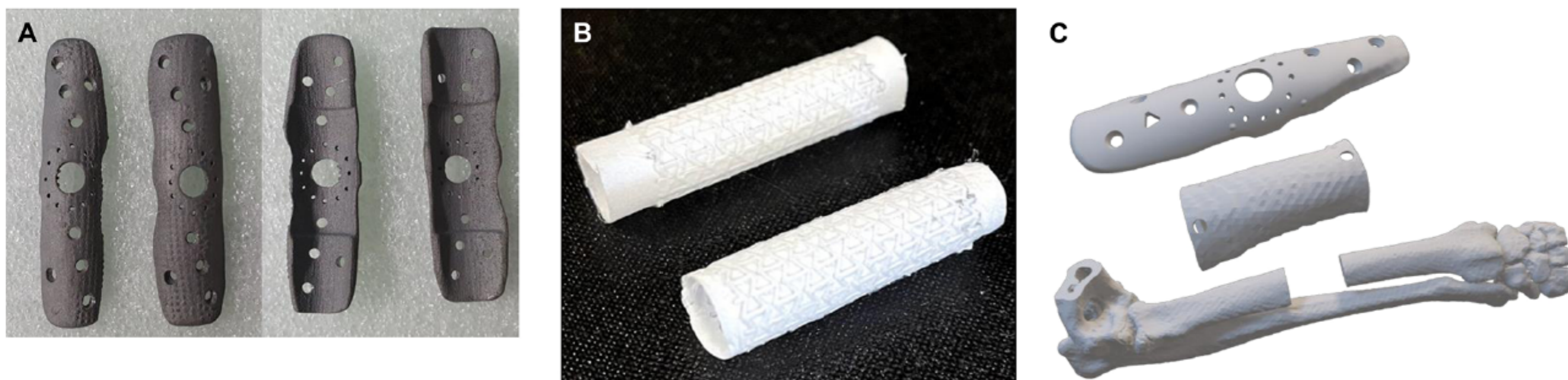
Fig. 1 Fabricated hybrid bone scaffold based on 3D printing. A Photograph of the porous titanium metal plate. B Photograph of the biodegradable polymer tube. C Schematic illustration of the 3D-printed scaffold tailored for bone regeneration in a beagle defect model
