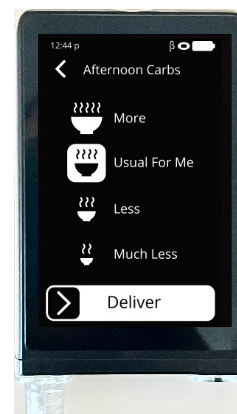
Figure 1. The iLet® Bionic Pancreas is initiated by inputting only the participant's weight. The user triggers mealtime insulin making a rough comparison of the coming meal's carbohydrate content to the carbohydrate of a usual meal for them (Usual for Me, More, or Less).
