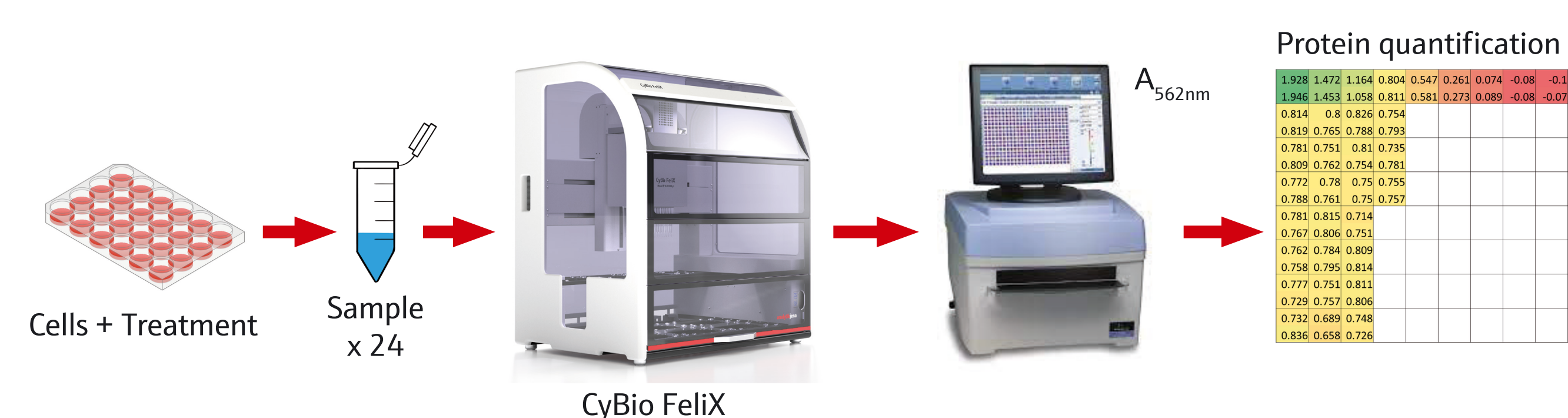
Figure 2 | Schematic of sampling and protein quantification. Total protein from cell lysate was quantified via BCA assay. The assay was prepared by the CyBio FeliX, the obtained protein concentration information was used to normalize samples during PROTAC assay setup.
