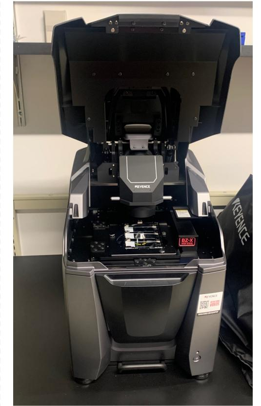
Figure 3. KEYENCE BZ-X800 Microscope used to NCAM expression. capture and stitch images sections.
