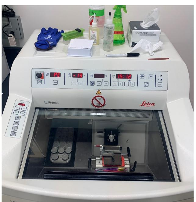
Figure 2. Cryostat machine that is used to slice skeletal muscle into cross-section and mount it onto glass slides.
