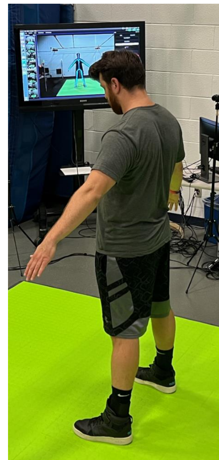
Figures 1 & 2 Illustrations of acquiring the image using the 3-D markerless motion capture system evaluated in the present study.
