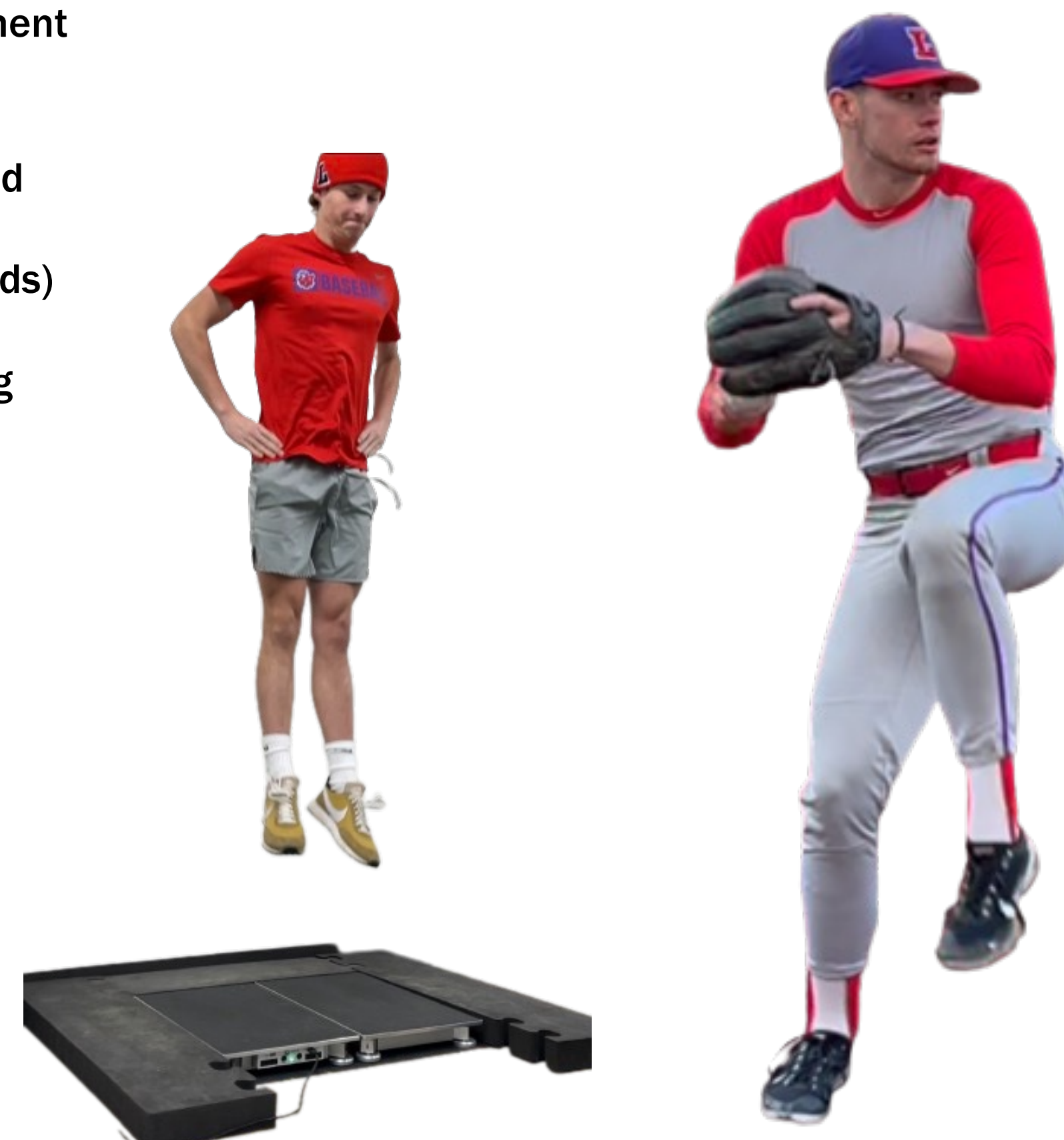
Figure 2: Countermovement jumps were collected through Hawkin Dynamics dual force plate system.
