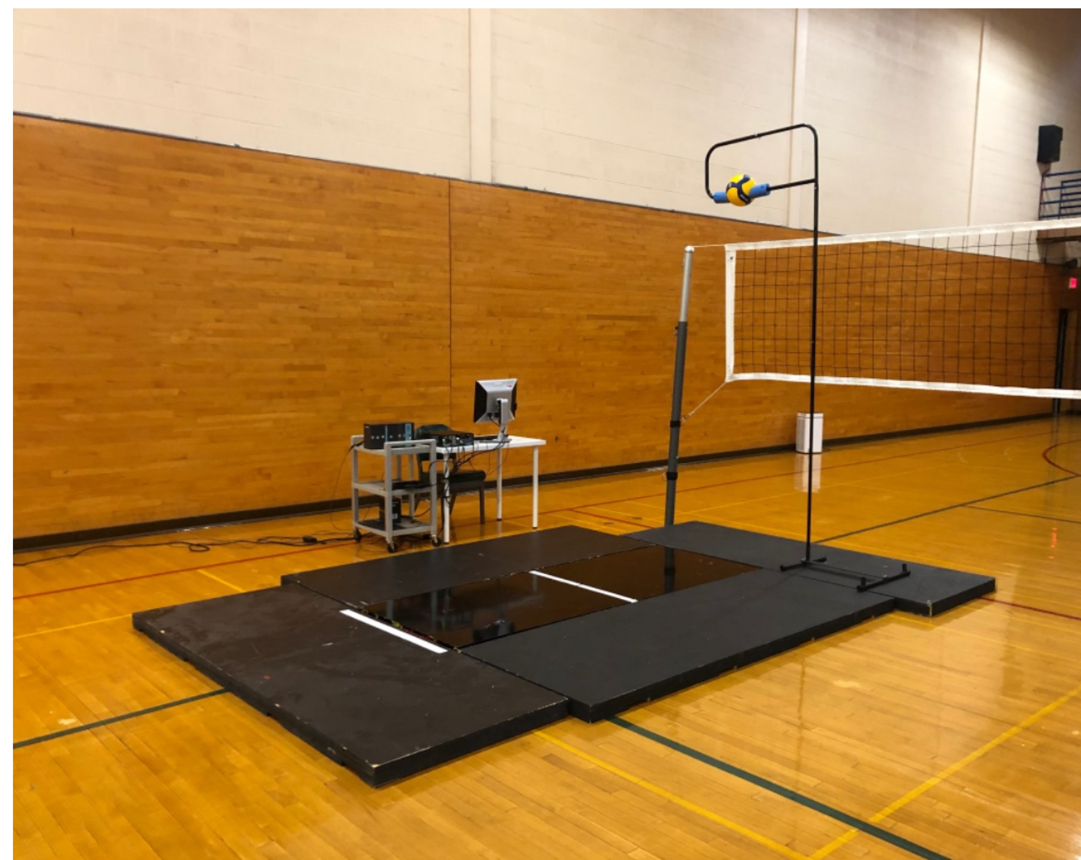
Figure 1. Graphical representation of the testing set-up including uni-axial force plate and attacking target positioned at 2.64 m.
