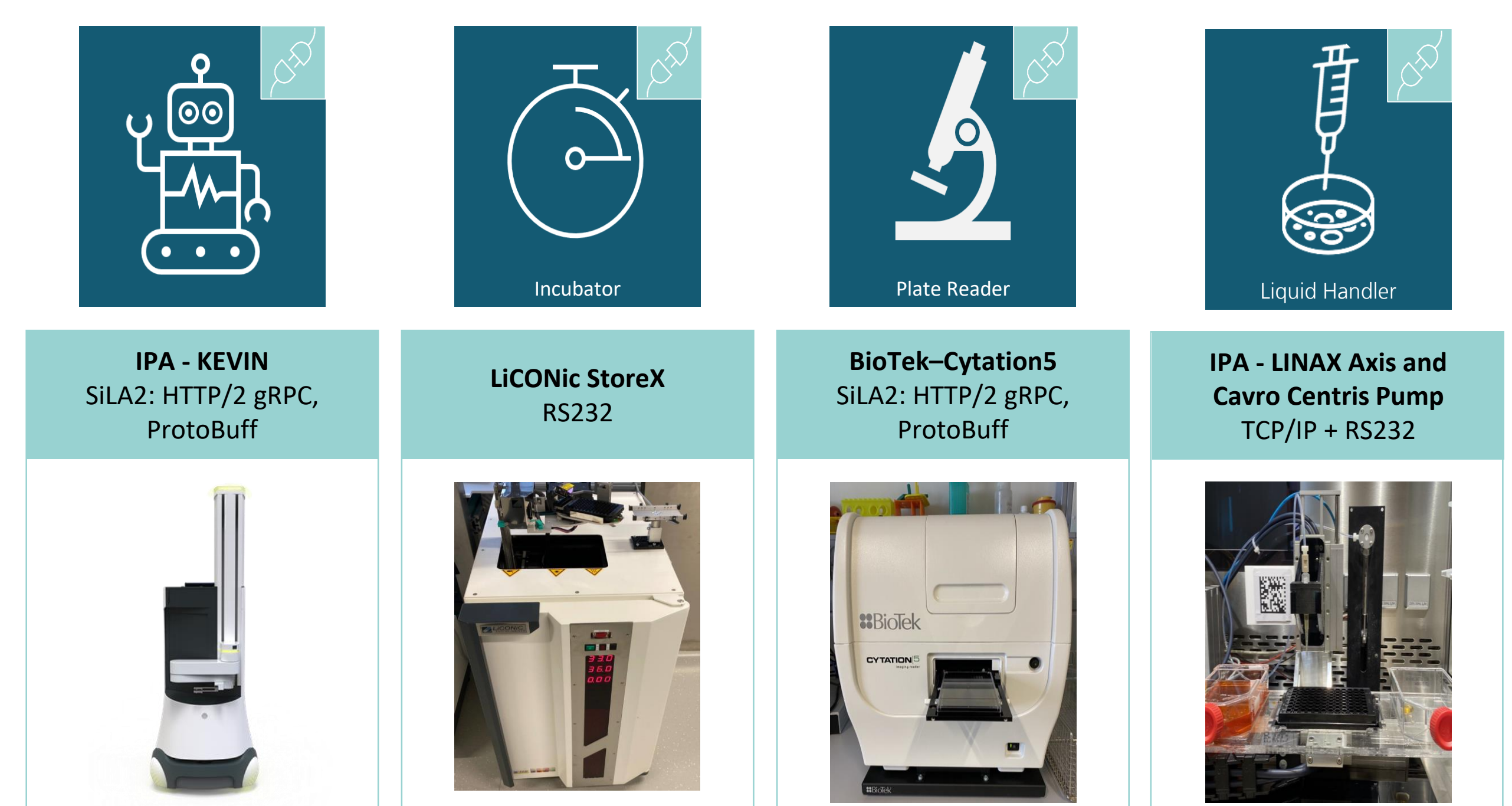
Figure 3: Integrated equipment used as an example for the media exchange use case
