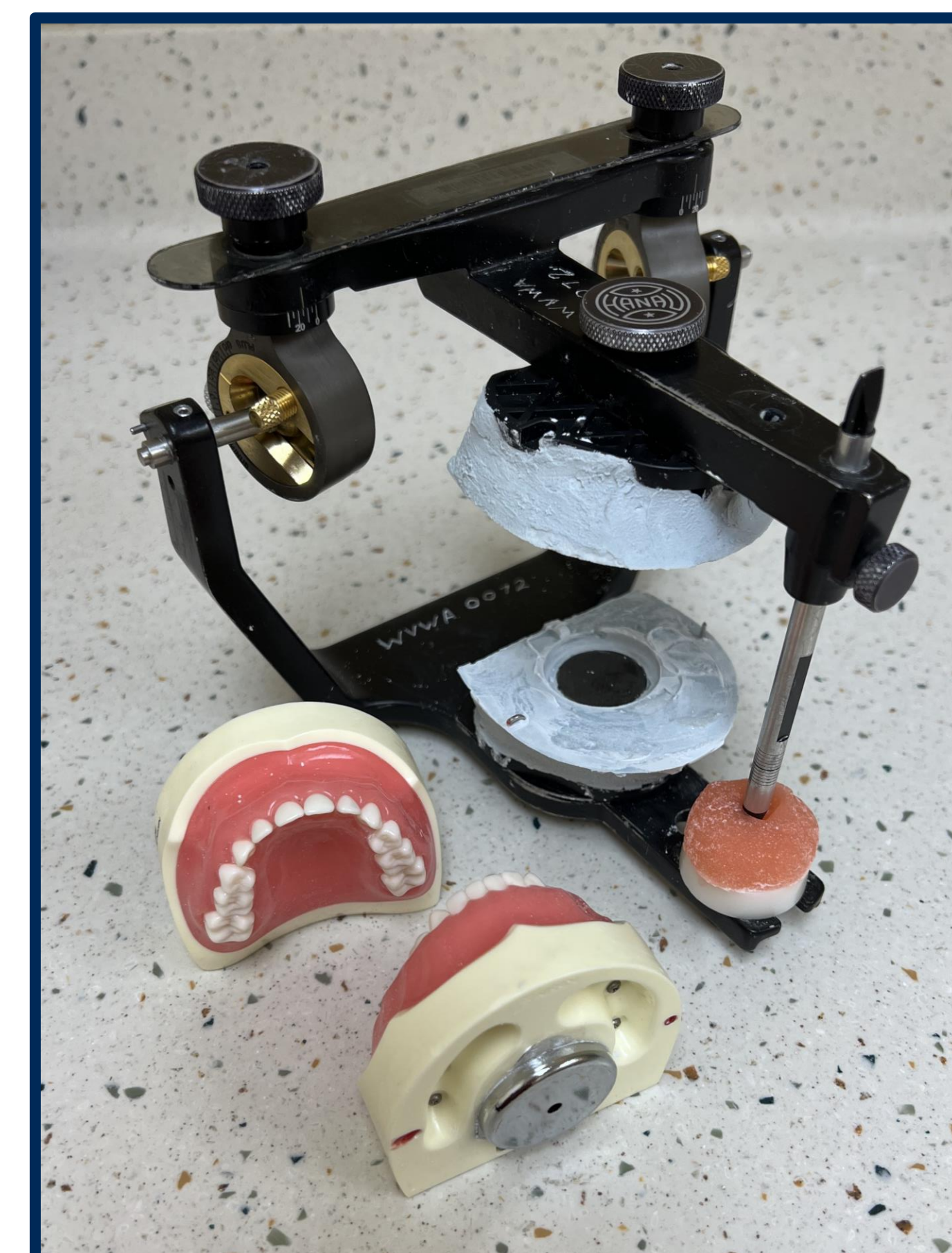
Figure 2: Articulator with Custom Incisal Guide Table
