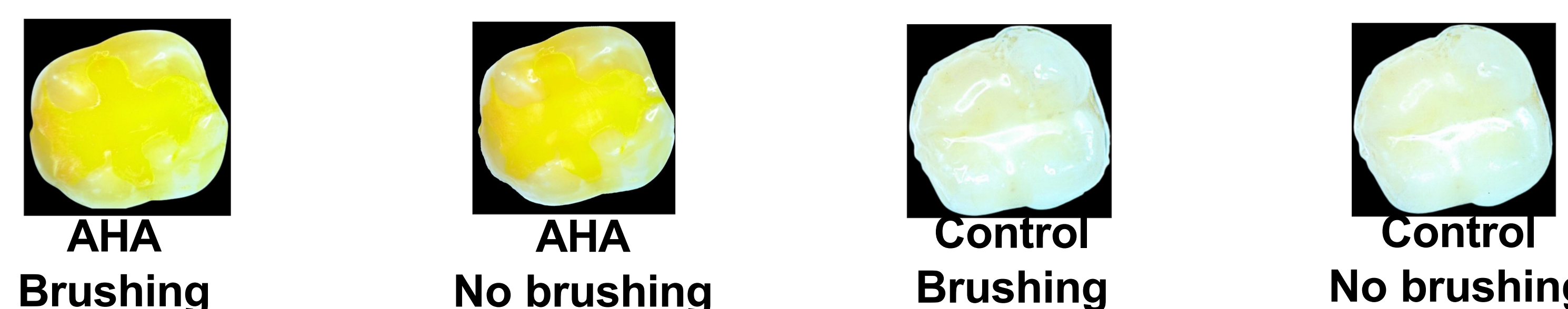
Figure 2: Photographs of substrates with dental sealants (control) or with AHA coating (test) with or without six months of simulated tooth brushing.
