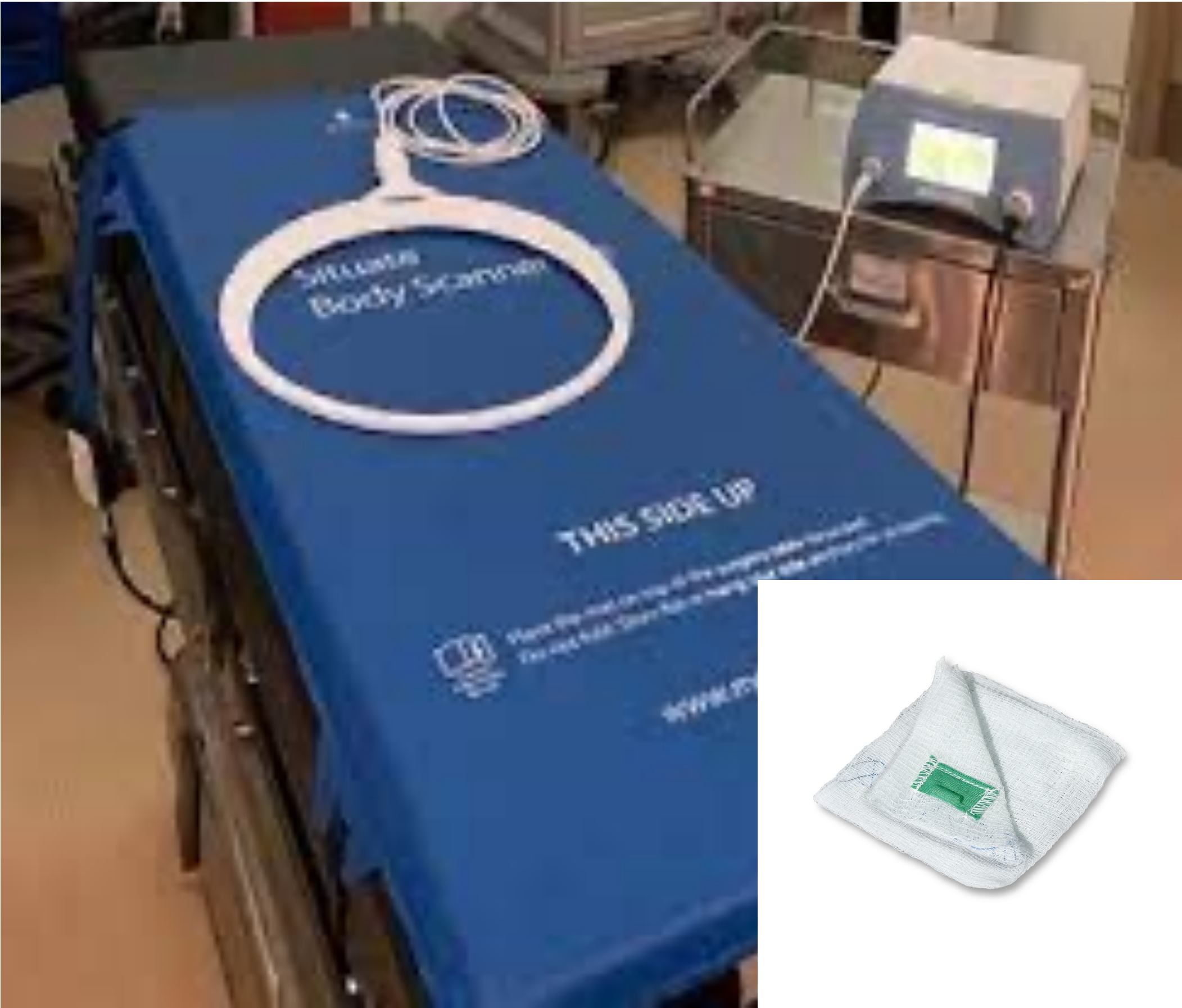
(Center): The blue RFID body scanner is placed under the patient 15 . (Top left) the white wand is scanned over the patient and is connected to the gray calibrating console (top right). The white tagged sponges are used during procedures (bottom right) 16 .
