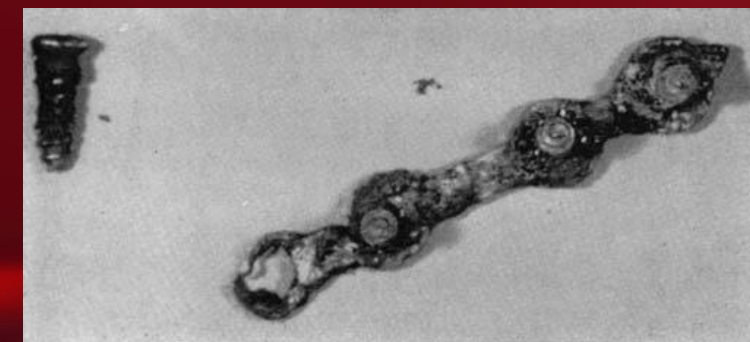
Figure 1 - Dr. Lane's original plate design showing signs of corrosion, 1959
